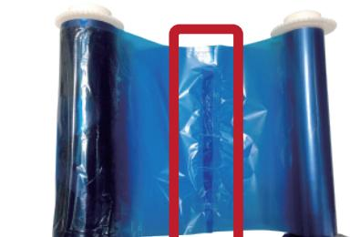
Tape the ribbon back together , and place ribbon back onto cartridge. Make sure to scroll the ribbon back onto the cartridge as tight as possible, till the broken part of the ribbon cannot be seen.
