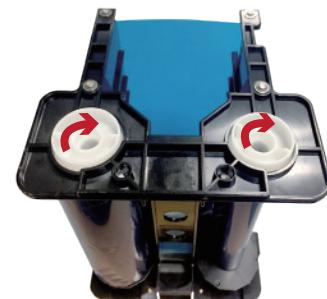
Press down on arrow indicated part, and scroll the ribbon as the arrow indicated, till the ribbon is as tight as possible on the cartridge.
